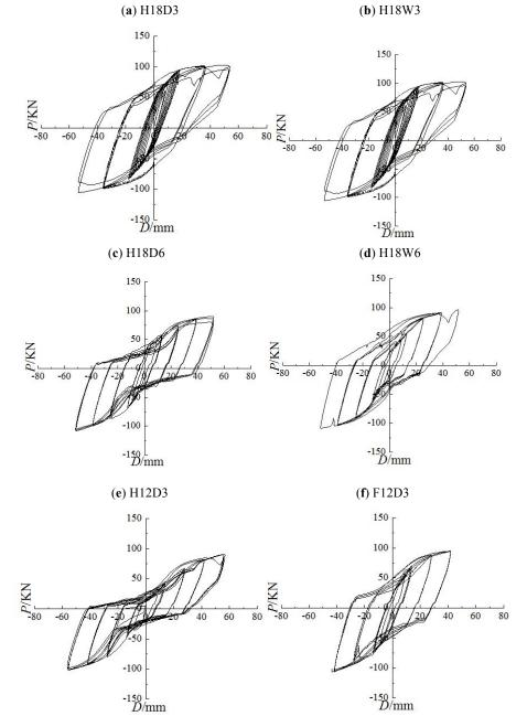
Fig. (5). Comparisons of P- $\Delta$  hysteretic curves of connection specimens.
