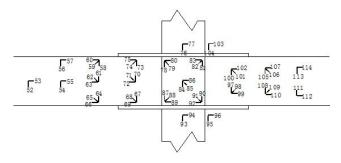
Fig. (3). Distribution of Strain gauges applied to the specimens.
