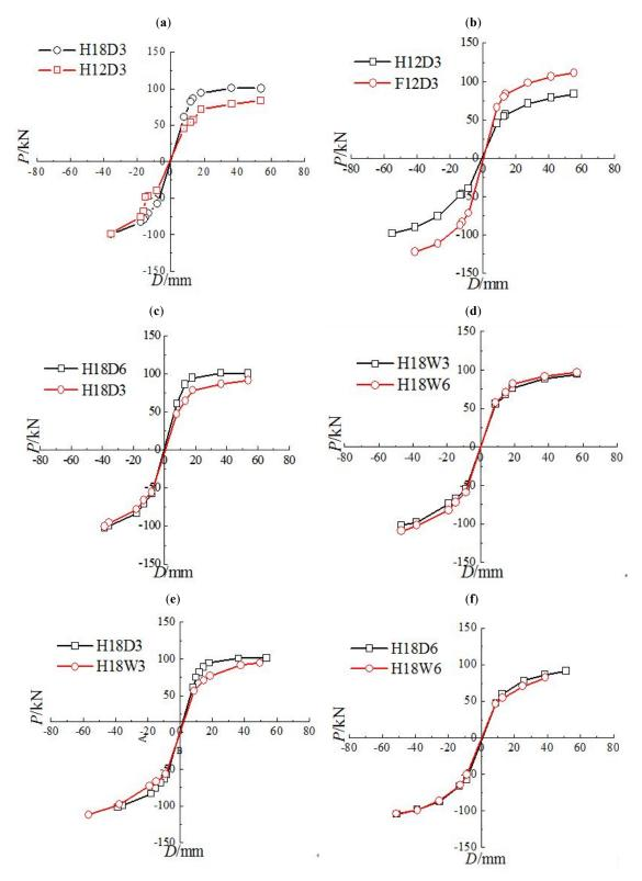
Fig. (6). Comparisons of P- $\Delta$  skeleton curves of connection specimens.
