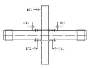
Fig. (4). Distribution of displacement transducers.
