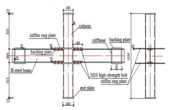
Fig. (1). Details of connection.
