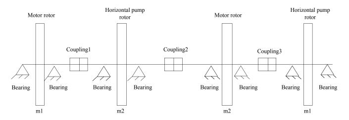
Fig. (2). Simplified model of amphibious disaster-resistant submersible pump with rotor system [5].
