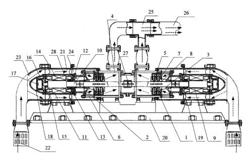
1 - Horizontal Pump; 2 - Coupling; 3 - Pump bearing; 4 - Water outlet; 5 - Mesomere; 6 - Suction; 7 - Guide vane; 8 - Impeller; 9 - Electric motor; 10 - Motor shaft; 11 - Motor case; 12 - Front housing; 13 - Mechanical seal device; 14 - Stator module; 15 - Rotor assembly; 16 - Thrust bearing; 17 - Adjust bag;
