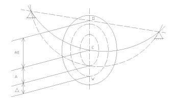
Fig. (3). Simplified model of horizontal pump with rotor system.
