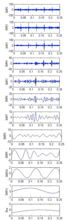
Fig. (3). EEMD decomposition results of broken-teeth signal.
