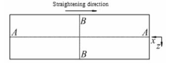
Fig. (5). The position of paths in the stainless steel clad plate.
