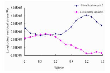
Fig. (7). Longitudinal residual stress path BB across width.
