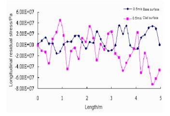
Fig. (6). Longitudinal residual stress path AA across length.
