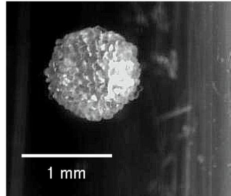
Fig. (6). Photograph of a bubble-particle aggregate completely loaded with silica particles of the coarser size distribution, rising in the quiescent aqueous solution of the viewing section.
