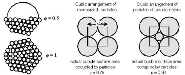
**Fig. (2).** Fraction of bubble surface area that adheres particles ( $\phi$ ) and fraction of bubble surface area actually occupied by particles ( $\epsilon$ ), when spherical particles are accommodated in a square array on the bubble surface (note that for a size distribution of particles  $\epsilon \rightarrow 1$ ).
