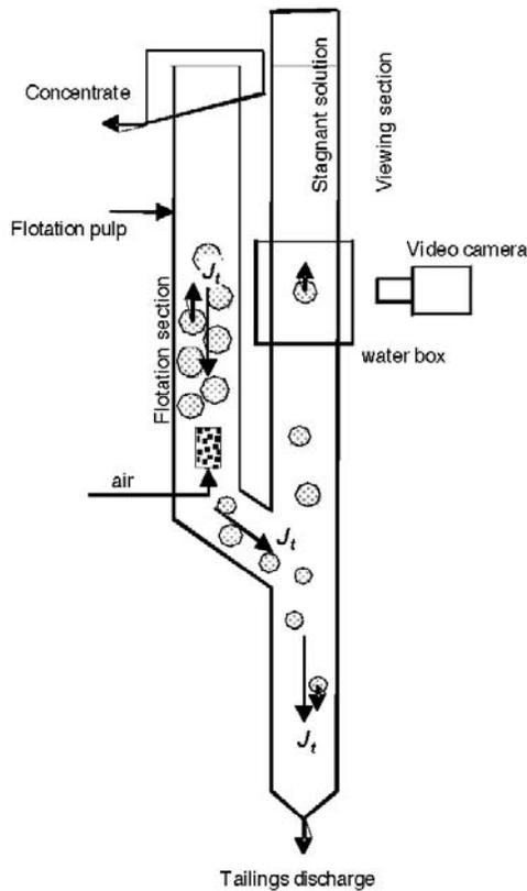
**Fig. (1).** Schematic of the modified flotation column used in this work, which illustrates the phenomenon under study and the experimental methodology used to measure the diameter and velocity of the bubble-particle aggregates that are dragged to the tailings discharge. ( $J_t$  is the slurry superficial rate, that is, the volumetric slurry flow rate divided by the cross-sectional area of the column).
