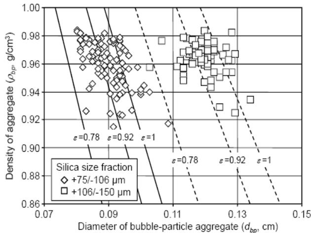
**Fig. (8).** Comparison between the relationship  $\rho_{bp}$  vs.  $d_{bp}$  obtained with the hydrodynamic model (symbols) and the geometrical model: full lines for the +75/-106  $\mu\text{m}$  size fraction and dashed lines for the +106/-150  $\mu\text{m}$  size fraction.
