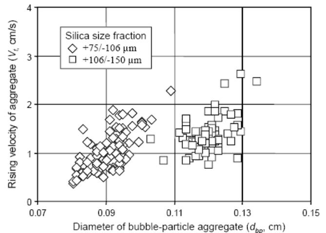
Fig. (7). (a) Terminal velocity of the bubble-particle aggregate ( $V_t$ ) vs. aggregate diameter ( $d_{bp}$ ), experimentally measured for the two silica size fractions tested.
