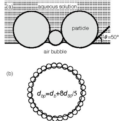
**Fig. (3).** Contact angle of  $50^\circ$  between particles and bubbles considered in the geometrical model, typical of moderately hydrophobic particles. It is proposed that the diameter of the particles seating on the bubble surface is the  $d_{80}$  of the distribution.
