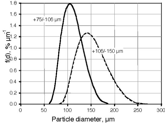
**Fig. (4).** Mass density function [10] of the silica sand used in this work, obtained with a Coulter LS100Q particle size analyzer based on laser diffraction techniques. The 80 percent passing size of the distributions ( $d_{80}$ ) are 118 y 161  $\mu\text{m}$ , for the size fractions +75/-106 and +106/-150  $\mu\text{m}$ , respectively.
