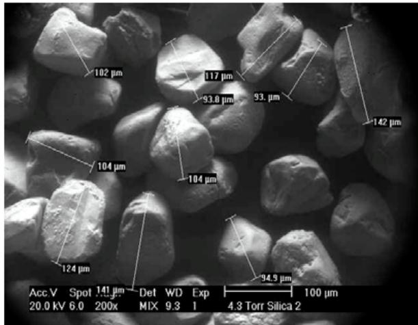
Fig. (5). Morphology of the silica sand used in this work, showing the rounded shape of the particles.
