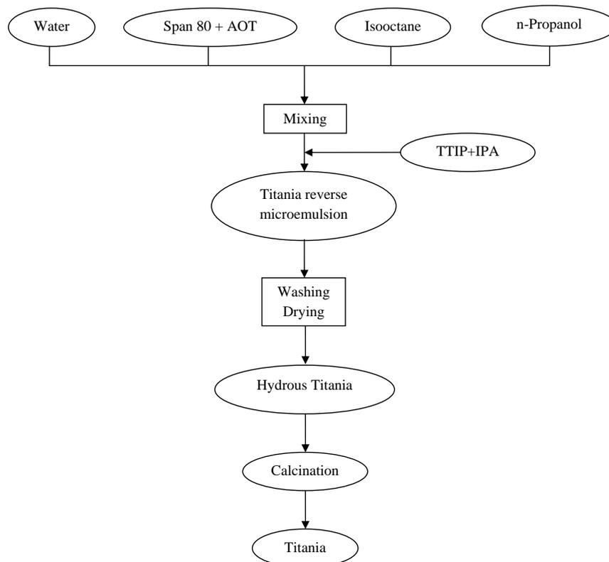
Fig. (1). Flow-Chart for nanosized titania powder preparation.
