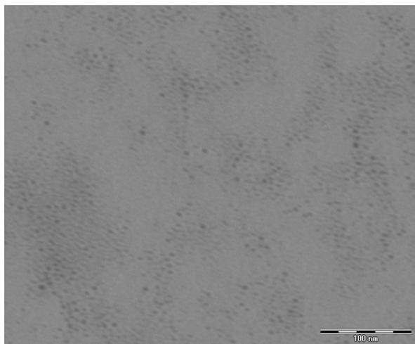
**Fig. (3).** TEM microphotographs of calcined sample prepared at water to surfactant ratio ( $w_0 = 4$ ).
