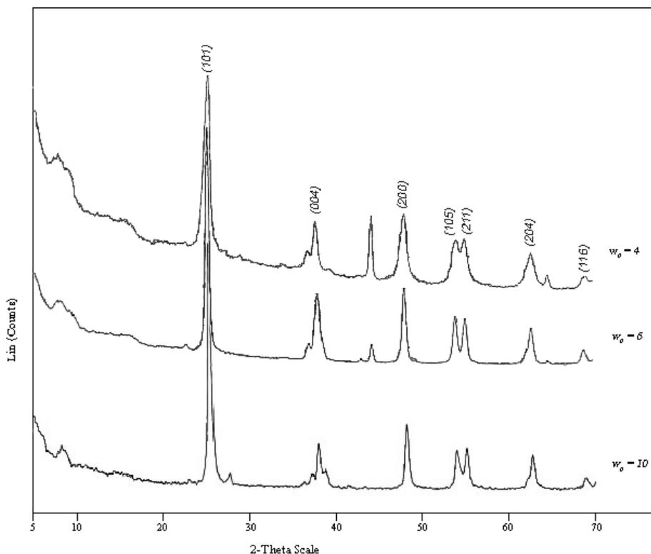
Fig. (2). XRD patterns of nanosized titania particles obtained from mixed reverse microemulsions at various water contents.
