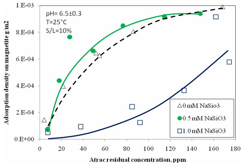
Fig. (9). Adsorption isotherms of Atrac on magnetite in the presence of water glass (WG).
