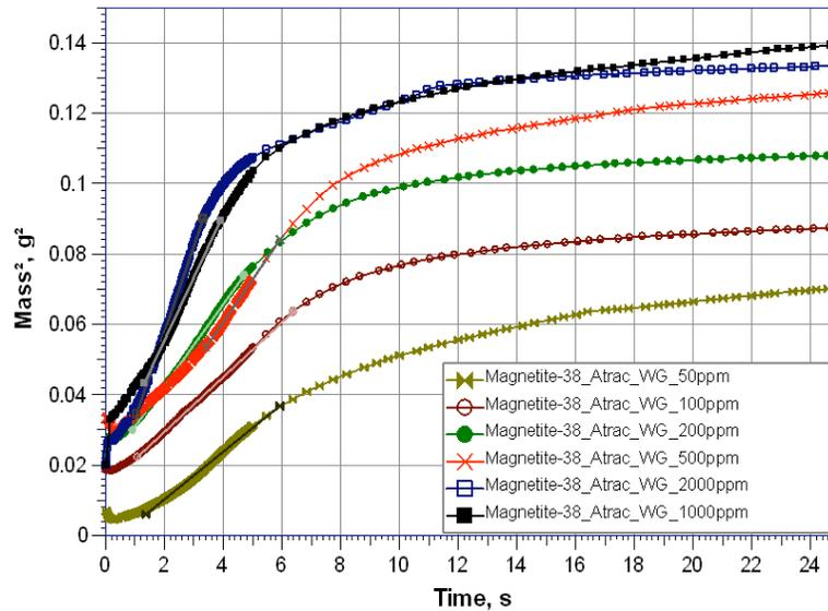
**Fig. (3).** Effect of sodium silicate (WG) concentration on water sorption of -38  $\mu\text{m}$  magnetite particles in the presence of 100 ppm Atrac collector.
