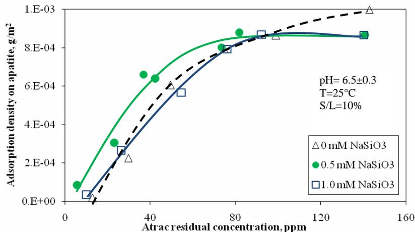
Fig. (8). Adsorption of Atrac on apatite in the presence of water glass (WG).
