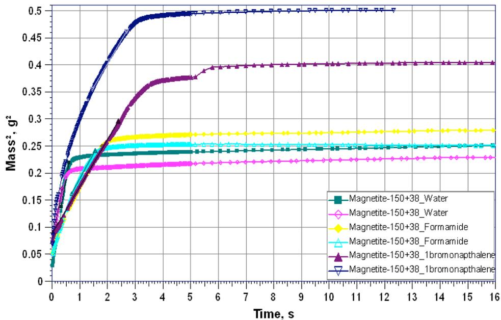
Fig. (1). Sorption curves of test liquids on magnetite for the measurement of contact angle.
