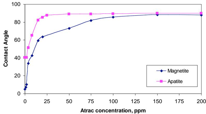
Fig. (4). Effect of Atrac concentration on water contact angle of -38  $\mu\text{m}$  magnetite and apatite particles.
