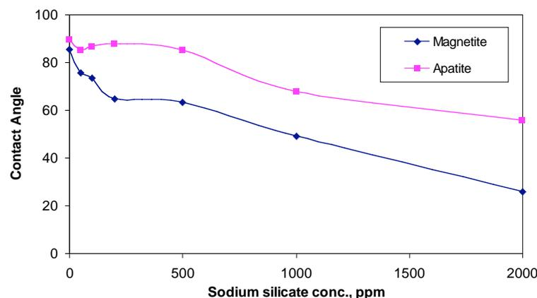
Fig. (5). Effect of sodium silicate concentration on water contact angle of -38  $\mu\text{m}$  apatite and magnetite particle in the presence of 100 ppm atrac collector.
