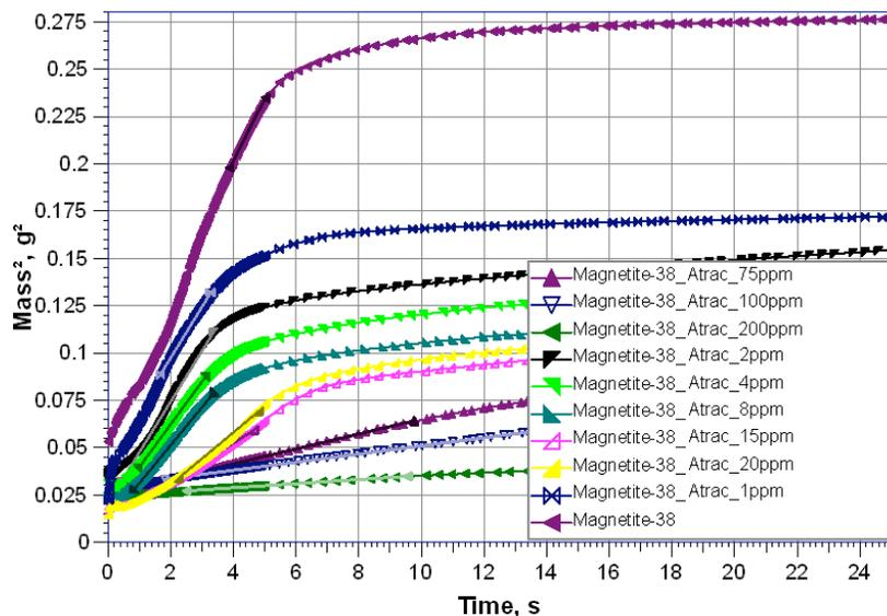
Fig. (2). Effect of Atrac concentration on water sorption of - 38 μm magnetite particles.
