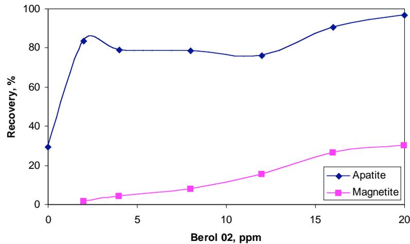
Fig. (13). Influence of non-ionic collector concentration on Atrac flotation of apatite and magnetite at 8.5 pH and 2 ppm Atrac.
