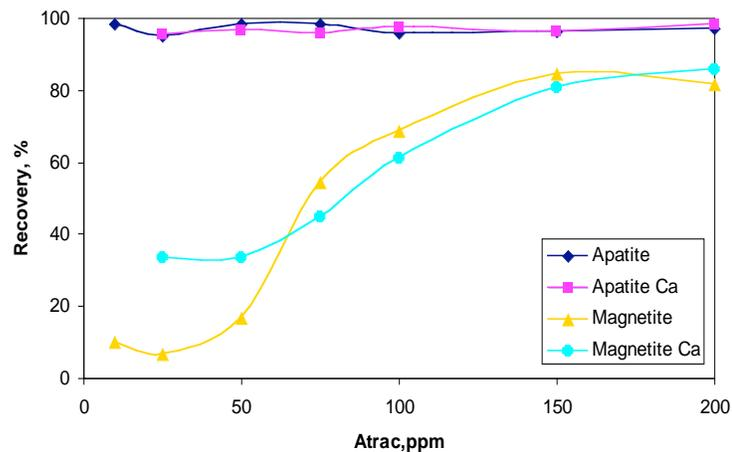
Fig. (10). Atrac flotation of apatite and magnetite in the presence and absence of calcium ions at 8.5 pH.
