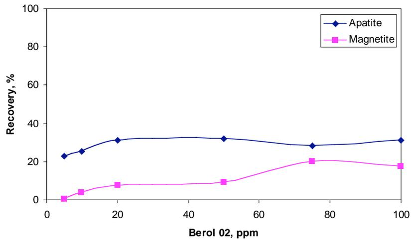
Fig. (12). Non-ionic collector flotation of apatite and magnetite at 8.5 pH.
