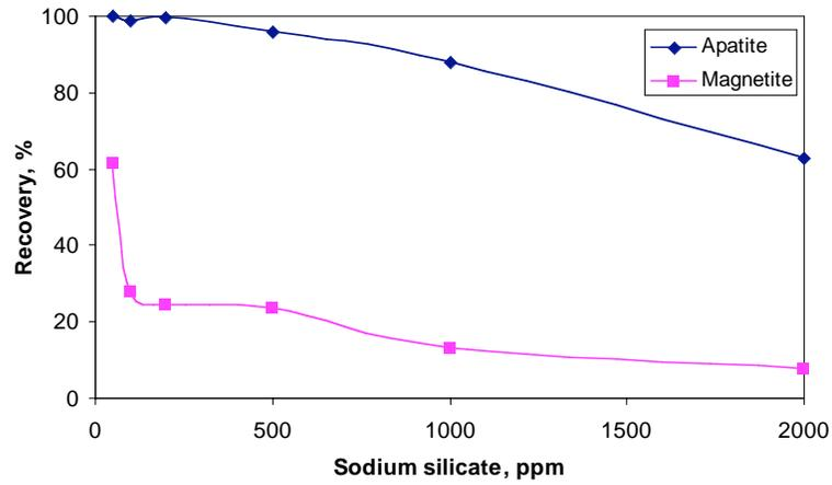
Fig. (11). Effect of water glass on Atrac flotation of apatite and magnetite at pH of 8.5 and 100 ppm Atrac.
