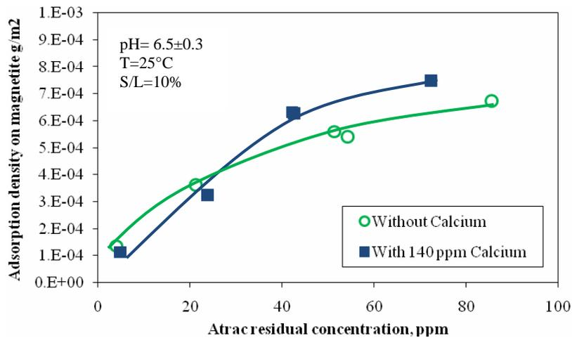
Fig. (7). Adsorption of Atrac on magnetite as a function of equilibrium concentration.
