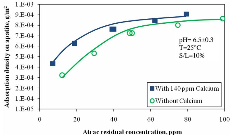
Fig. (6). Adsorption of Atrac on apatite as a function of equilibrium concentration.
