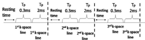
**Fig. (2).** *diagonal-SPRITE* multi-T<sub>p</sub> acquisition approach. After a short resting time the same lines of k-space is detected at two different T<sub>p</sub> (in this diagram only two T<sub>p</sub> have been used T<sub>p</sub>= 0.3 ms and T<sub>p</sub>= 2 ms). The process is repeated for all the k-space lines.
