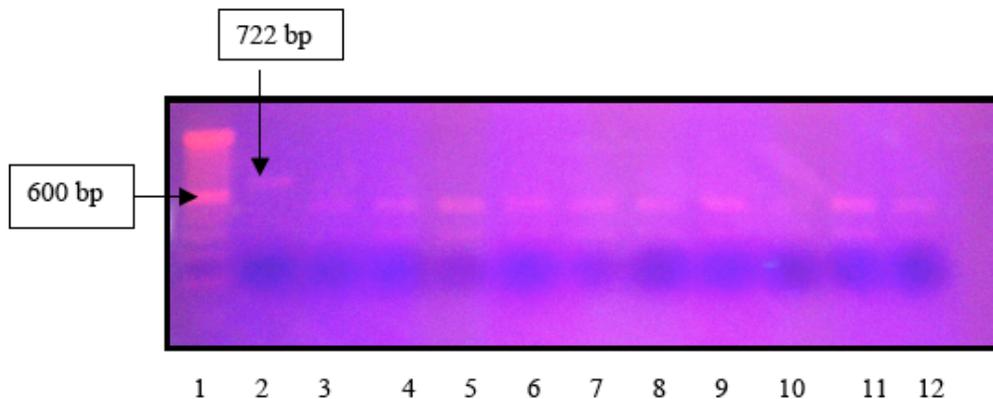
Fig. (2). Restriction enzyme analysis of PCR product by Apal enzyme. Lane 1= DNA marker, lane 2= Single band of PCR product (control sample) with no enzyme (722 bp), and lane 3-12= double bands of wild type samples cutting by Apal enzyme.
