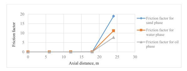
Fig. (3). Friction factor for sand, oil and water along the axial distance.
