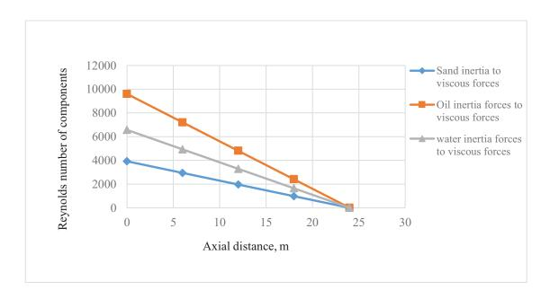
Fig. (4). Reynolds number of components along the axial distance.
