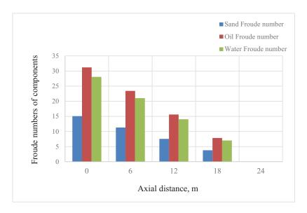
Fig. (6). Froude number of oil, sand and water along the axial distance.
