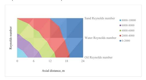
Fig. (2). Reynolds number of sand, oil and water at different times along the axial distance.
