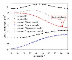
Fig. (12). The safe mud weight window vs. well inclination at azimuth of N30 $^{\circ}$ E.
