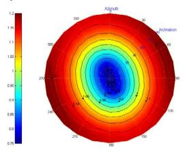
**Fig. (8).** Critical collapse pressure vs. well azimuth with depleted pore pressure (our model with horizontal stress reorientation).
