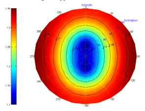
**Fig. (6).** Critical collapse pressure vs. well azimuth with original pore pressure.
