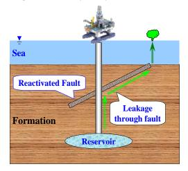
**Fig. (1).** Fault reactivation when drilling near the fault (Oilfield in Bohai Bay Basin).
