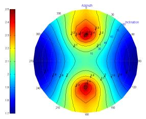
**Fig. (7).** Critical fracture pressure vs. well azimuth with original pore pressure.
