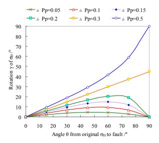
Fig. (3). Rotation angle ( $\gamma$ ) of horizontal stress orientation vs. the included angle ( $\theta$ ) between fault strike and original orientation of  $\delta_{H}$ .
