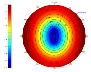
**Fig. (10).** Critical collapse pressure vs. well azimuth with depleted pore pressure (the previous model neglecting horizontal stress reorientation).
