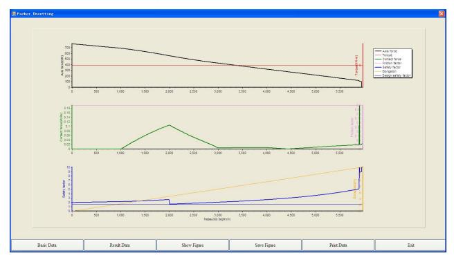
Fig. (5). Mechanical conditions of T-1 well string in packer unsetting.
