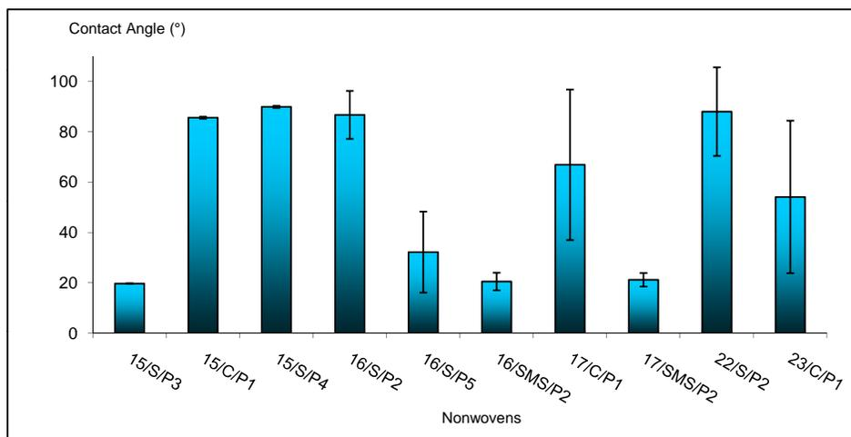
Fig. (5). The contact angle for different nonwoven fabrics.
