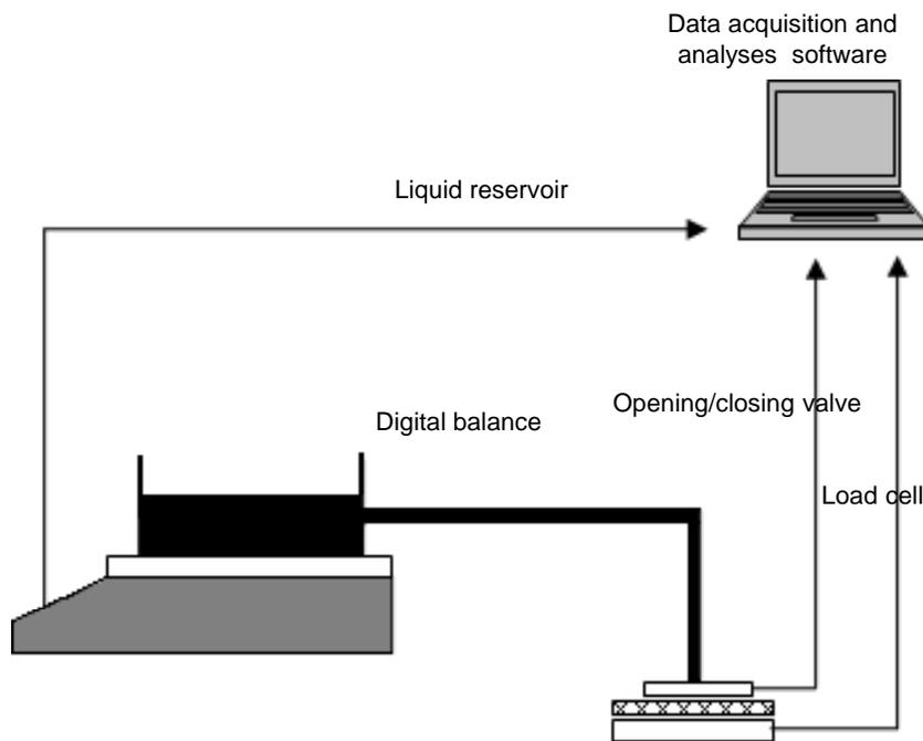
Fig. (3). Schematic diagram of absorption kinetics measurement.
