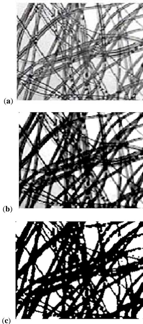
**Fig. (2).** Image transformation process to nonwoven image: (a) original image, (b) filtered image and (c) binary image.
