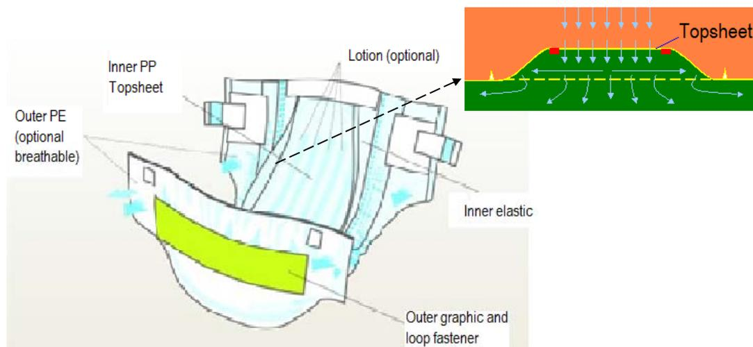
**Fig. (1).** Schematic overview of a modern disposable diaper.
