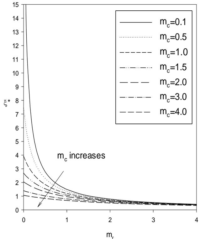
**Fig. (18).** Fin Optimum Effectiveness  $\xi^*$  vs.  $m_r$  with  $m_c$  Varying  $n=0.0, R_w=1.0, \theta_e=0.5, C=10$ .
