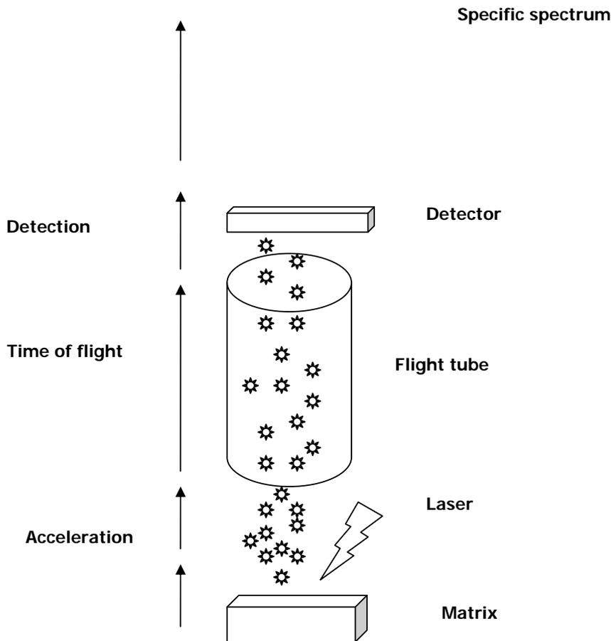
**Fig. (1). Principles of MALDI-TOF MS technique.** The samples are first inserted and embedded in a matrix. A laser pulse is applied in the matrix and the molecules are then both desorbed and ionized by charge transfer. The molecules are accelerated in an electrical field passing through a flight tube and collide with a detector. Biomolecules are separated according to their mass. Finally, a mass spectrum is created which is compared with a database for the identification of the virus.
