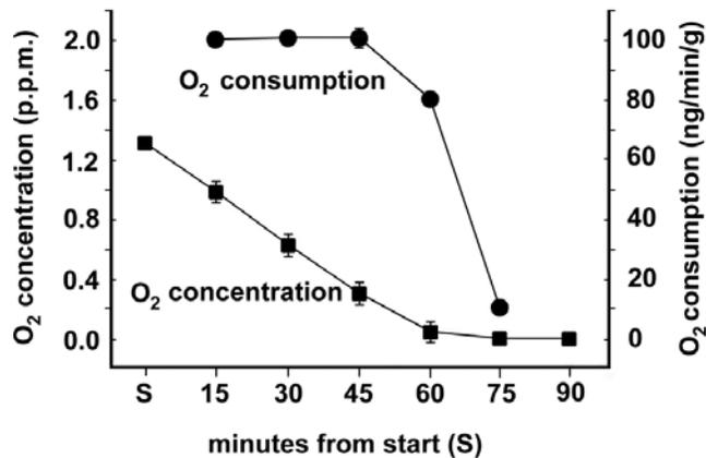
**Fig. (2).** Oxygen concentrations in the respiratory chamber (small squares) in parts per million (ppm), recorded every fifteen minutes during hypoxic treatment, and oxygen consumption of the newts (circles) in ng/min/g. Each point represents the mean from eight readings; the vertical bars indicate the standard deviations. S: start of experiment.
