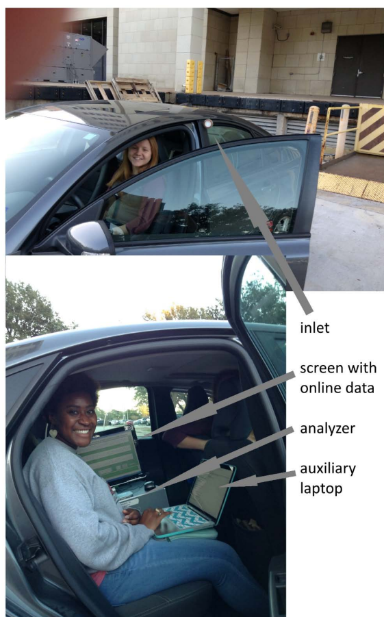
Fig. (1). Mobile study setup - top picture showing undergraduate student Kristen Koch, driving most routes and recording position, and the gas inlet out the left rear window; bottom picture showing undergraduate student Shelby Thomas monitoring the measurements and taking auxiliary notes. Not visible is the power supply, a 12 VDC lead acid battery placed behind the driver seat.
