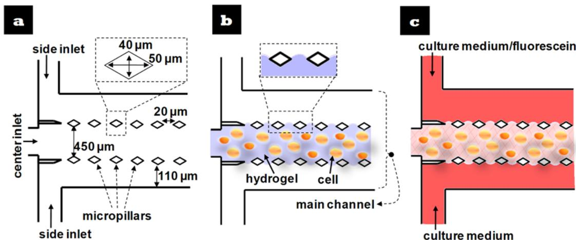
**Fig. (1).** Schematic procedure for fabricating a stripe-shaped hydrogel matrix. (a) A microfluidic device having diamond-shaped micropillar arrays in the middle of the main channel of a MMA device (b) Hydrogel containing cells is flowed *via* center inlet of the main channel. Any kinds of hydrogels can be patterned. (c) Culture medium or drug solution is flowed *via* both sides of inlets.
