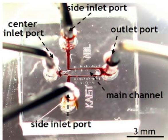
**Fig. (2).** A fabricated microfluidic micropillar arrays (MMA) device.
