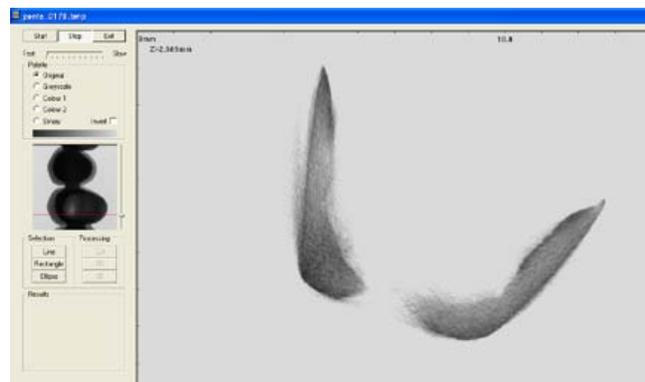
**Fig. (2).** The Micro-CT 3D images provided evidences of corrosion and structural defects in the micro architecture of the prostheses obtained from the patient. (A) dental appliance obtained from the patient. (B) a new dental appliance.
