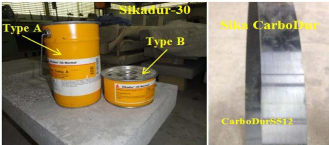
Fig (3). Manufactured forms of CFRP materials.
