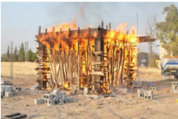
Fig. (2). Reinforced concrete frame exposed to fire.
