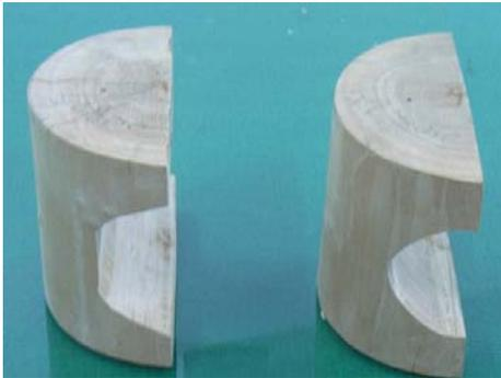
Fig. (2). Wooden models of trapezoid and arc joints
