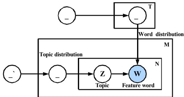
Fig. (1). Representation of LDA model.
