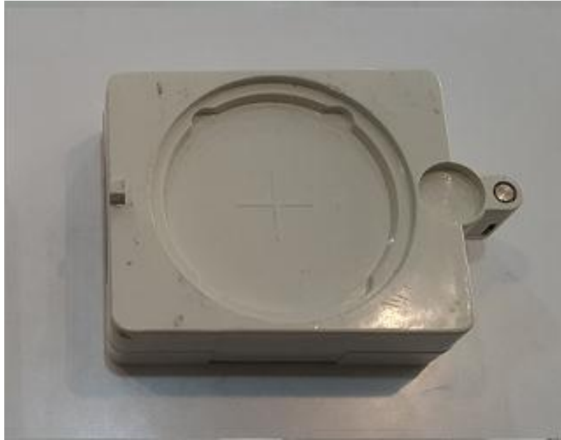
Fig. (1). Phantom (for evaluating density and spatial resolution).
