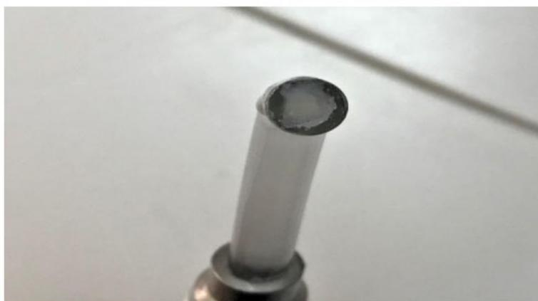
Fig. (1). A layer of composite residue covering most of the tip of one LCU as received before cleaning.
