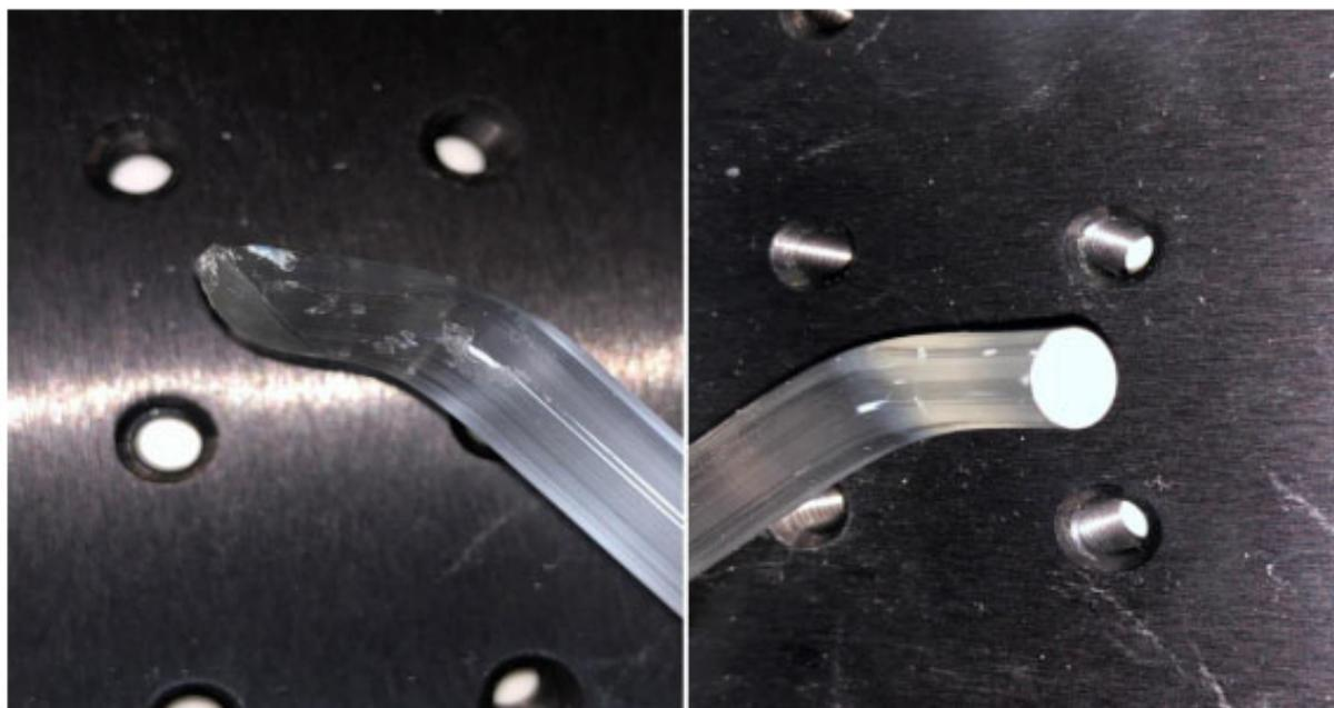
Fig. (2). Shows a damaged tip for (Acteon mini LED) versus a new tip.
