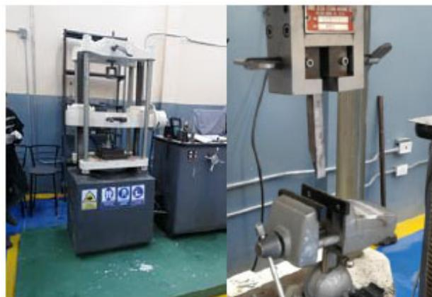
Fig. (5). Universal testing machine and appearance of the chisel used for shearing of the brackets.
