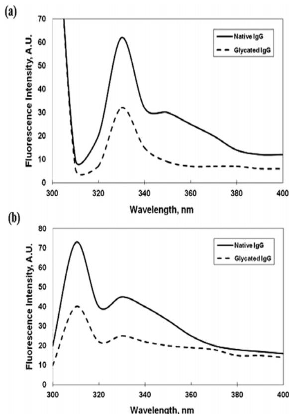
**Fig. (2).** Fluorescence emission spectra of native (—) and AGE-modified (---) IgG. Protein was in PBS, pH 7.4 at a concentration of 1.5  $\mu\text{M}$ . The excitation wavelength was 295 nm (a) and 280 nm (b). The spectra are the average of three determinations.
