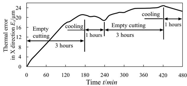
Fig. (4). Thermal errors in X-axis direction.
