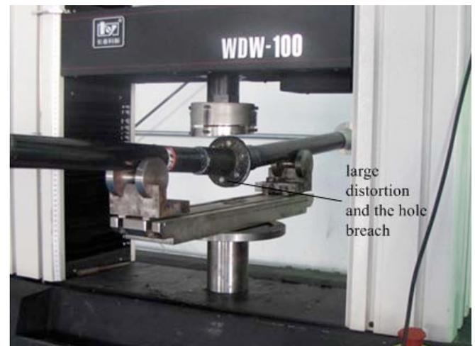
Fig. (12). Destroy of the composite material flange by the bending test.
