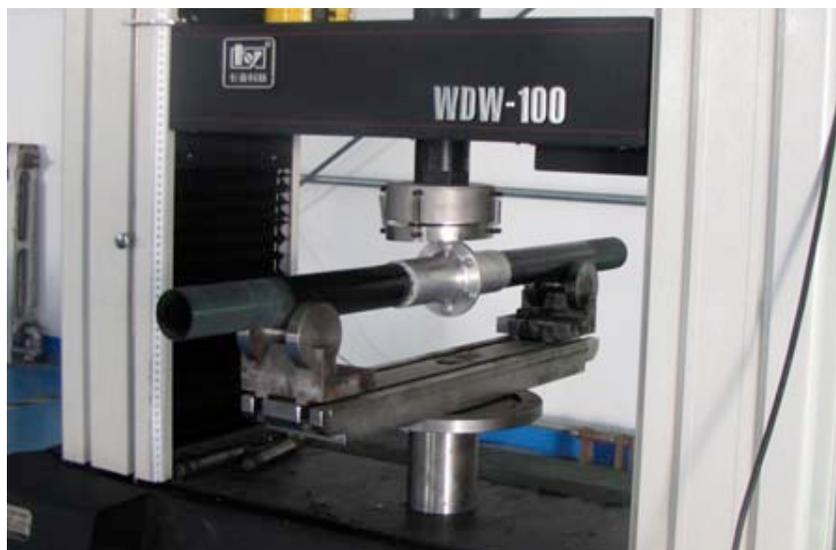
Fig. (17). Aviation aluminum alloy flange bending test.
