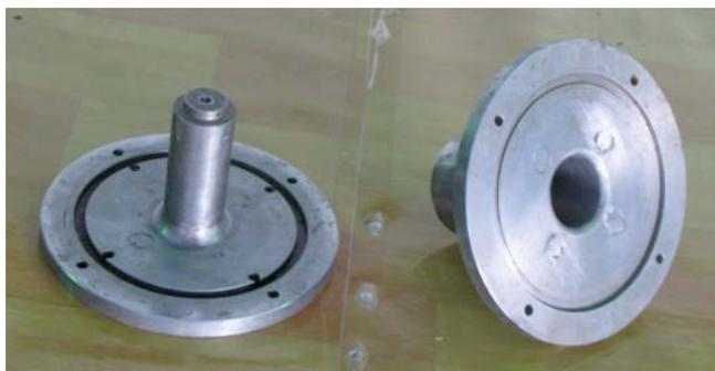
**Fig. (6).** Photos of the male mold and the female mold.
