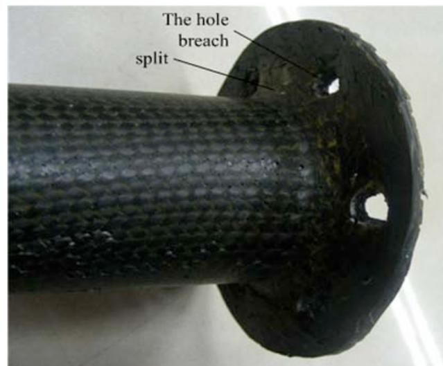
**Fig. (9).** Destroy of the composite material flange by the tensile test.
