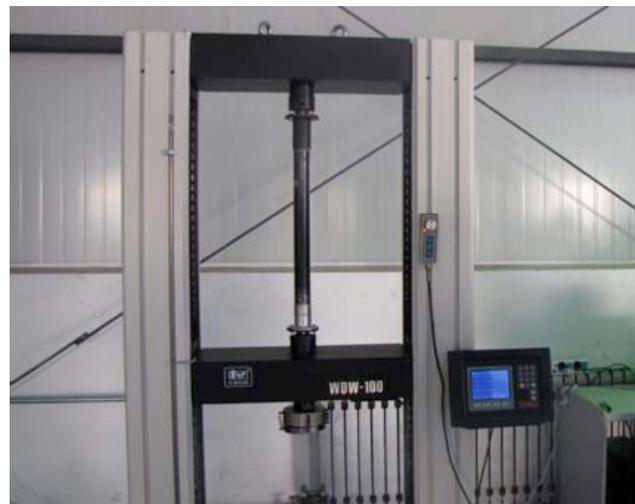
**Fig. (8).** Composite material flange tensile test.
