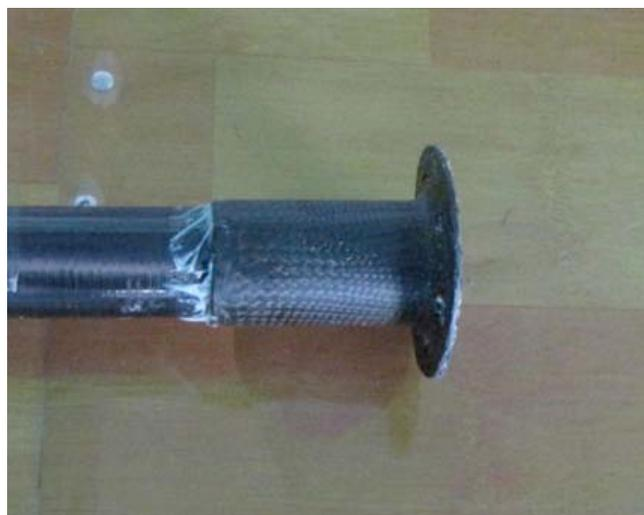
**Fig. (7).** Advanced composite material flange.
