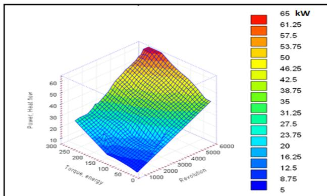
Fig. (1). The engine heat map for cooling system.
