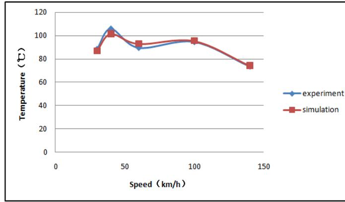
Fig. (5). The coolant of radiator temperature.
