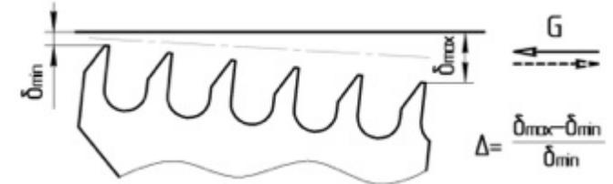
Fig. (5). Taper seal value.
