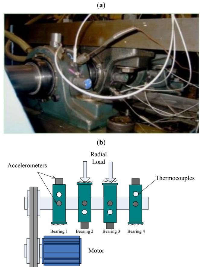
Fig. (9). Bearing fatigue test. (a) Test bench (b) Sketch map of bench.
