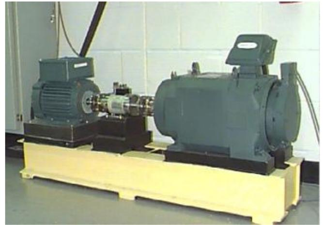
Fig. (5). Bearing fault simulation experiment table.
