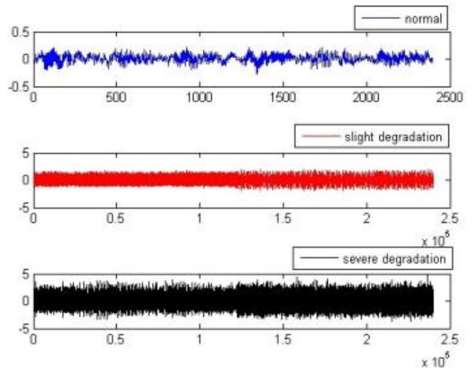
Fig. (6). Three fault degree of inner race.
