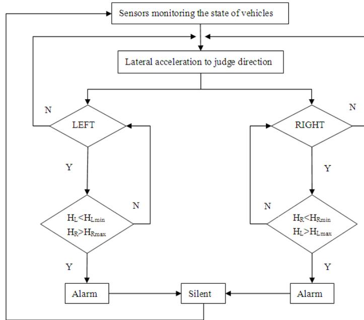
Fig. (1). The process of principle of rollover warning.
