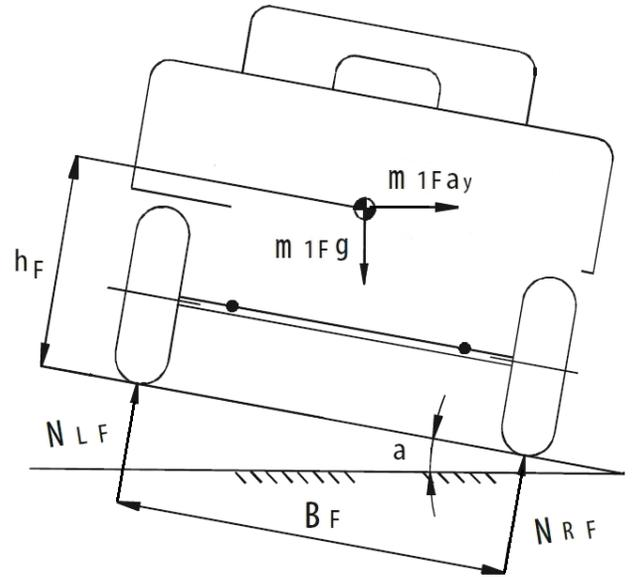
Fig. (3). The schematic diagram of force of front suspension spring force when turning right.
