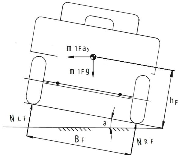
Fig. (2). The schematic diagram of force of front suspension spring force when turning left.
