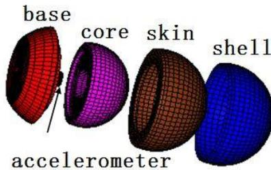
Fig. (2). Exploded view of child headform impactor.
