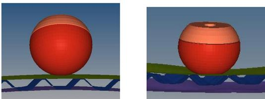
Fig. (8). The deformation view of the trapezium sandwich hood at collision point C3.
