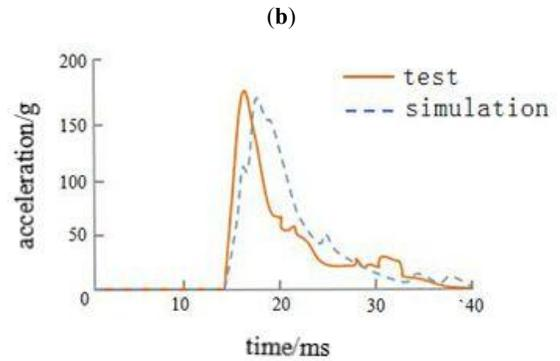
Fig. (3). Validation simulation (a) test setting (b) acceleration comparison of test and simulation.
