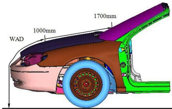
Fig. (1). Finite element model of the sedan front structure.
