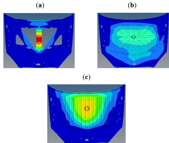
Fig. (9). The energy contours at collision point C3 (a) original structure (b) radial stiffener structure (c) trapezium sandwich.
