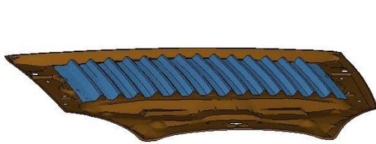
Fig. (7). The trapezium sandwich structure.
