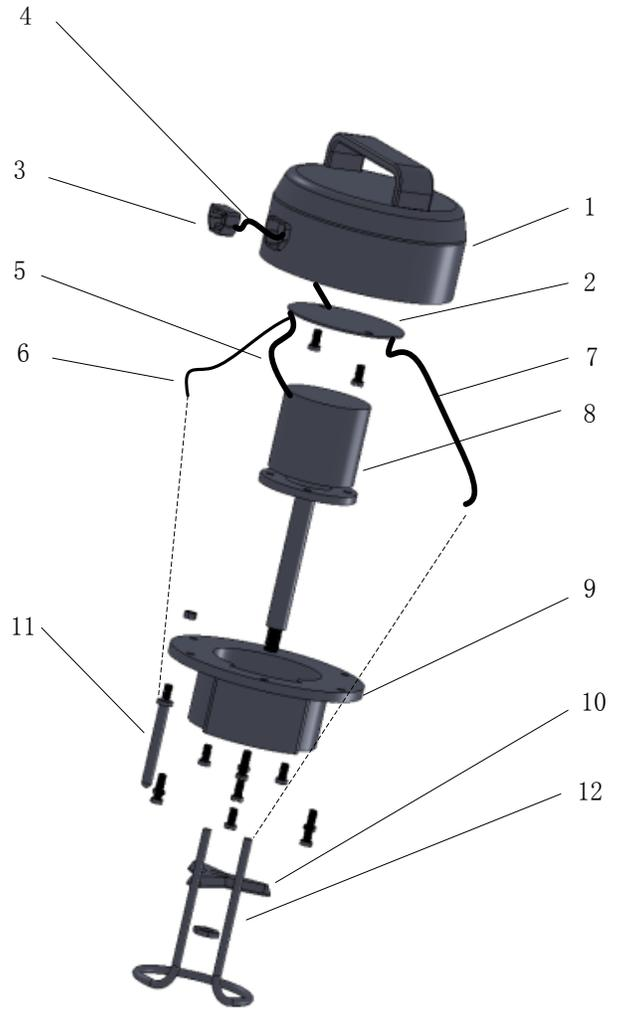
Fig. (7). Structure of head of soybean milk machine.
