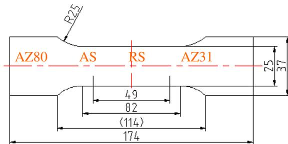
**Fig. (1).** Drawing of tensile sample.
