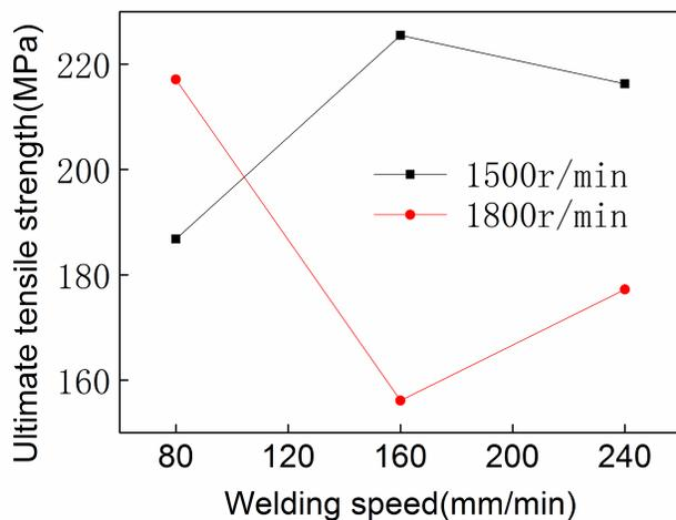
Fig. (5). Effects of FSW parameter on tensile strength.
