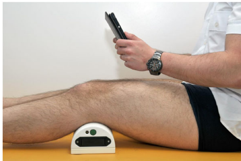
Fig. (2). Start position with training device directly underneath the subject's knee. The tablet is wirelessly connected to the device through a Bluetooth function.
