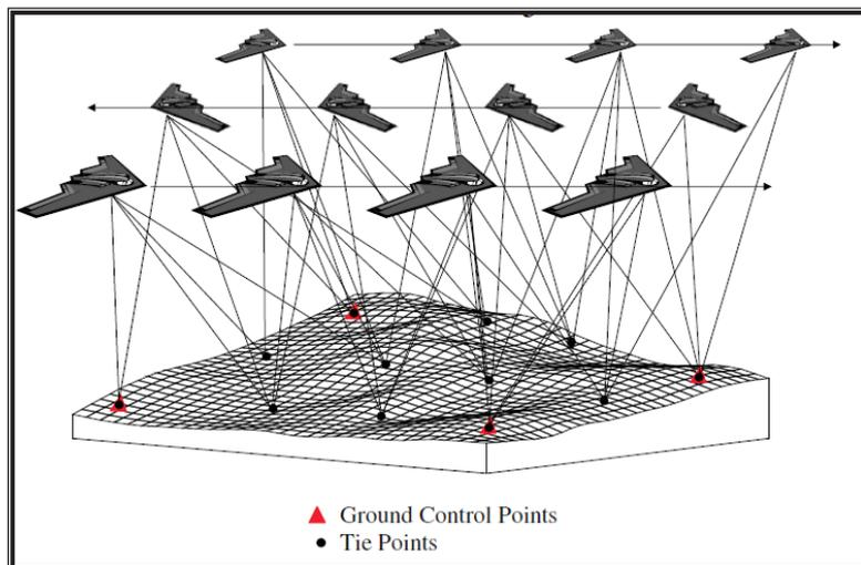
Fig. (4). Bundle block adjustment [8].
